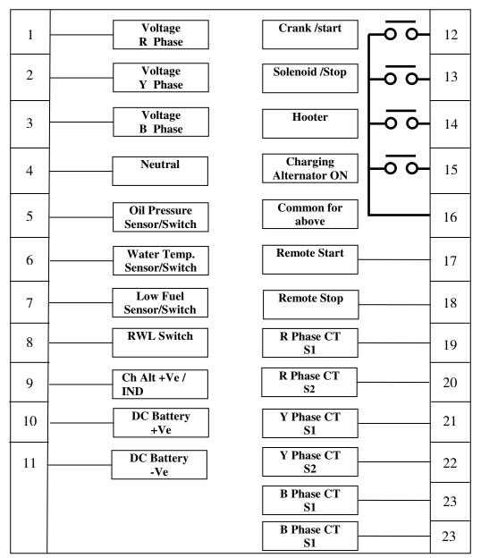
For single phase version Y&B Phase Voltages and Curent terminal are to be left open
