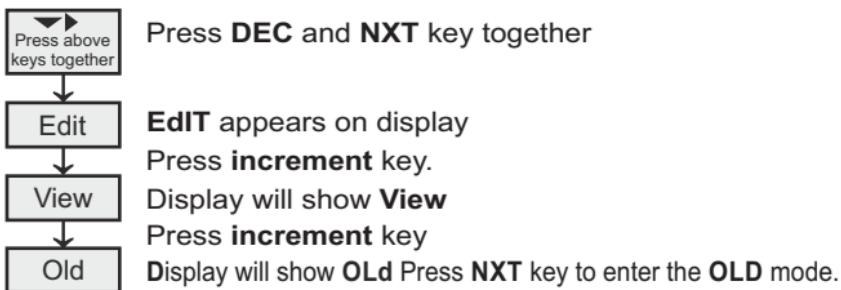
Each press of **NXT** key. To view old integrated parameter i.e KWH, KVAH, run hour, load hour, interruption which is model dependent
